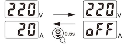
Under normal operation, the load can be switched on or off manually by pressing the power key for 0.5 seconds.
