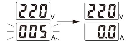
During the power-on and fault reset of the product, the product will count down and display according to the set delay time, and will enter the running state when the countdown ends.
